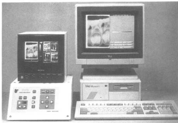
Figure 5. The RadioVisioGraphy system for direct digital dental imaging. The system consists of an intraoral charge-coupled device sensor and a processing unit with monitor.
